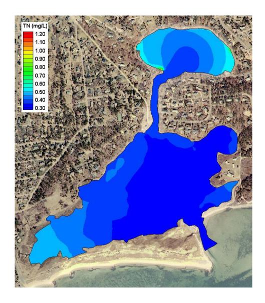
Contour Plot of **modeled total nitrogen concentrations**(**mg/L**) in the Taylors Pond/Mill
