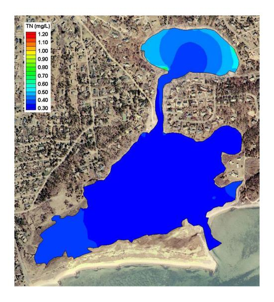
Contour Plot of **modeled total nitrogen concentrations** (**mg/L**) in the Taylors Pond/Mill Creek system, for present loading conditions.
