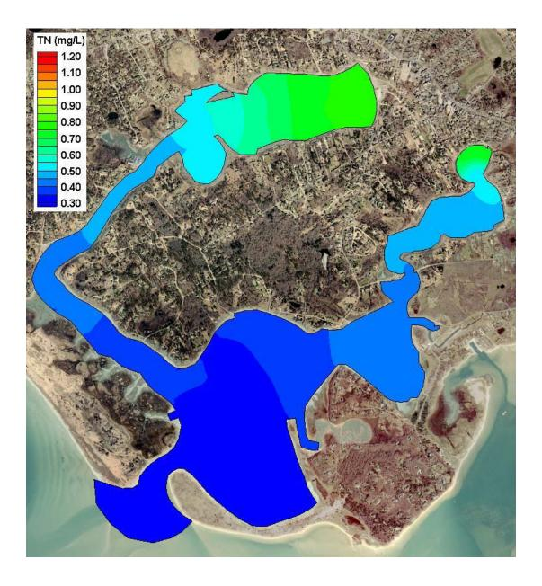
Contour Plot of **modeled total nitrogen concentrations** (**mg/L**) in the Stage Harbor system, for projected build out loading conditions.
