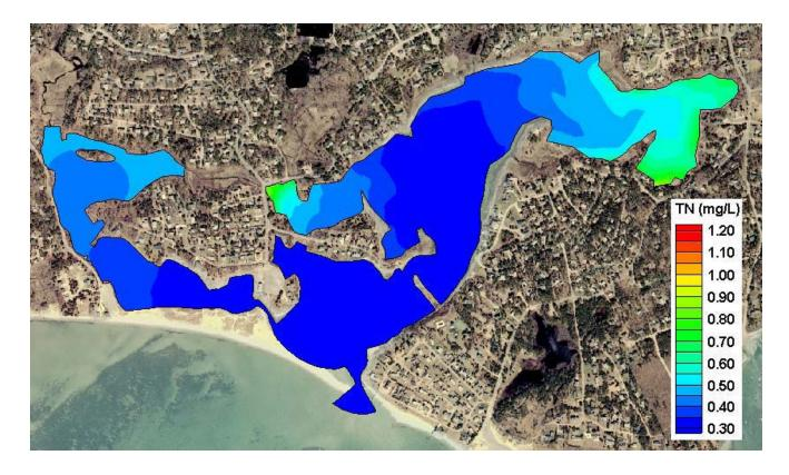
Contour Plot of modeled total nitrogen concentrations (mg/L) in the Sulphur Springs/Cockle Cove Creek system, for no anthropogenic loading conditions.
