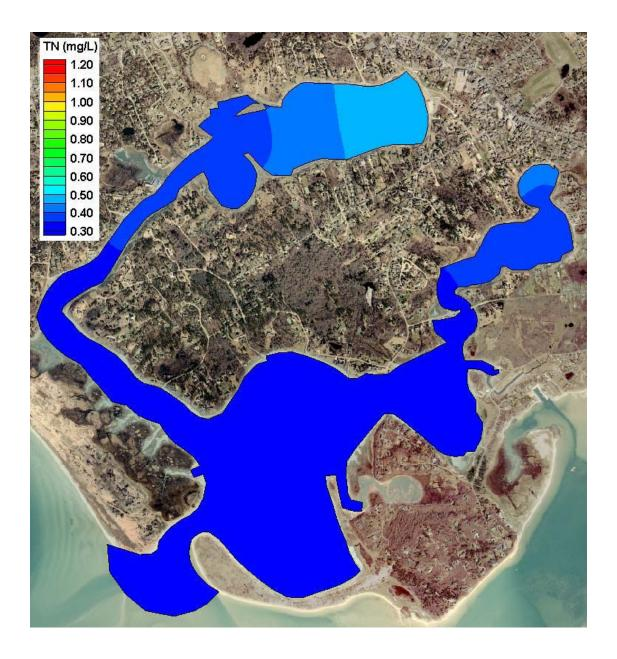
Contour Plot of modeled **total nitrogen concentrations** (**mg/L**) in the Stage Harbor system, for no anthropogenic loading conditions.
