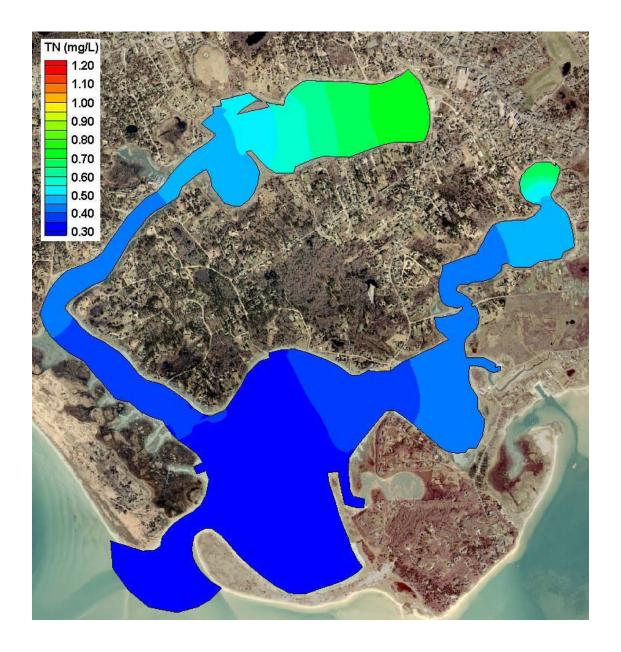
Contour plot of **average total nitrogen concentrations** from results of the present conditions loading scenario, for the Stage Harbor system.
