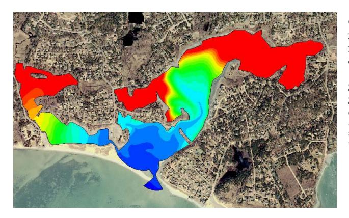
Contour Plot of modeled total nitrogen concentrations (mg/L) in the Sulphur Springs/Cockle Cove Creek system, for projected build out loading conditions
