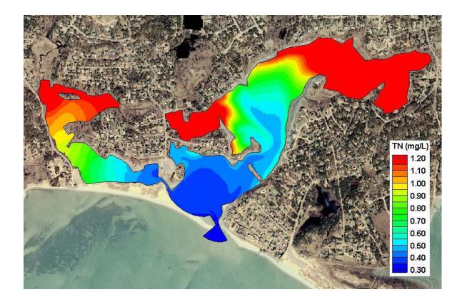
Contour Plot of modeled total nitrogen concentrations (mg/L) in the Sulphur Springs/Cockle Cove Creek system, for present loading conditions.
