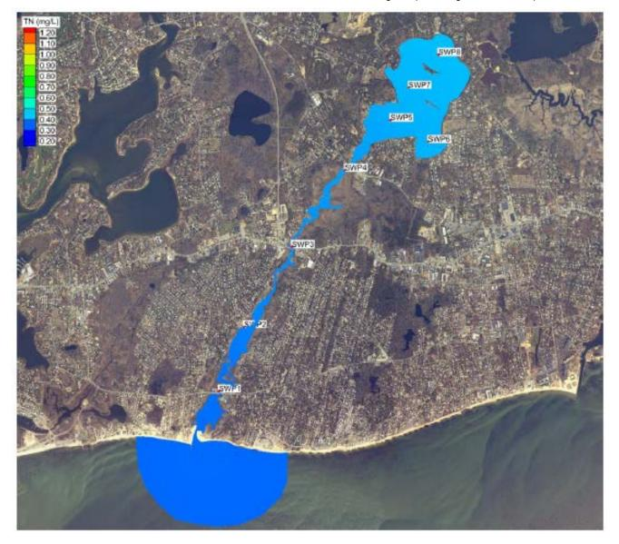
Contour Plot of modeled total nitrogen concentrations (mg/L) in Swan Pond River system, for no anthropogenic loading conditions, and bathymetry. The approximate location of the sentinel threshold station for Swan Pond River system (SWP-2) is shown.
