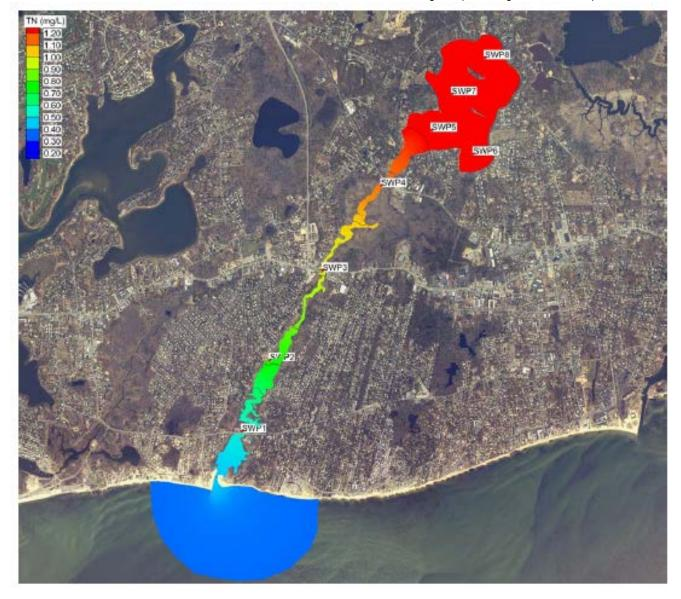
Contour plots of modeled total nitrogen concentrations (mg/L) in Swan Pond River system, for projected build-out loading conditions, and bathymetry. The approximate location of the sentinel threshold station for Swan Pond River System (SWP-2) is shown.
