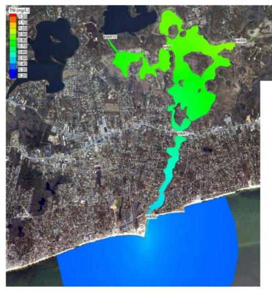
Contour Plot of average total nitrogen concentrations from results of the present conditions loading scenario, for Herring River System. The approximate location of the sentinel threshold station for Herring River System (HAR-7) is shown.
