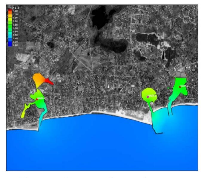
Contour plots of **modeled** total nitrogen concentrations (mg/L) in Allen Harbor. **Wychmere Harbor and** Saquatucket Harbor estuarine systems, for projected build-out loading conditions. The approximate location of the sentinel threshold stations for Allen Harbor (HAR-4), Wychmere Harbor (HAR-3), and Saquatucket Harbor (HAR-2) are shown.
