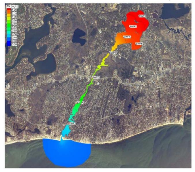
Contour Plot of average total nitrogen concentrations (mg/L) from the results of the present conditions loading scenario, for Swan Pond River system. The approximate location of the sentinel threshold station for Swan Pond River system (SWP-2) is shown.
