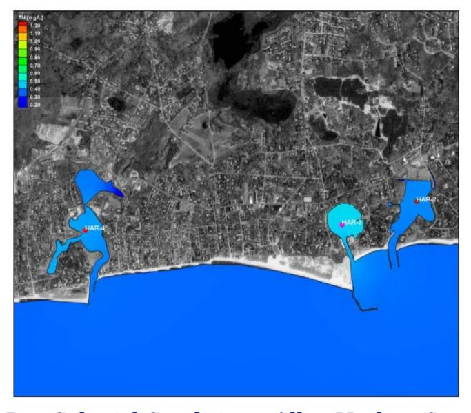
Contour Plots of **modeled** total nitrogen concentrations (mg/L) in the Allen Harbor. **Wychmere Harbor and** Saquatucket Harbor estuarine systems, for no anthropogenic loading conditions and bathymetry. The approximate location of the sentinel threshold stations for Allen Harbor (HAR-4), Wychmrere Harbor (HAR-3), and Saquatucket Harbor (HAR-2) are shown.
